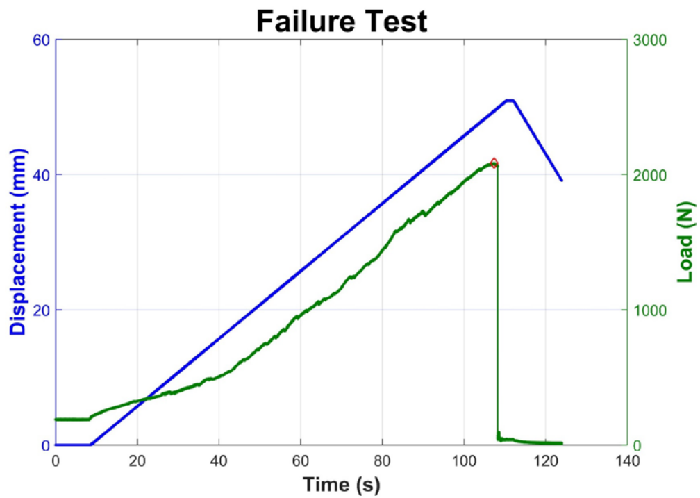
Figure 2 Quadriceps tendon displacement ramp of 0.5 mm/s and corresponding tendon loads with the knee fixed at 45° of flexion until patella fixation failure at 2084 N.
